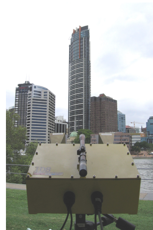
Fig. 2: IBIS-S in front of the hi-rise building.
