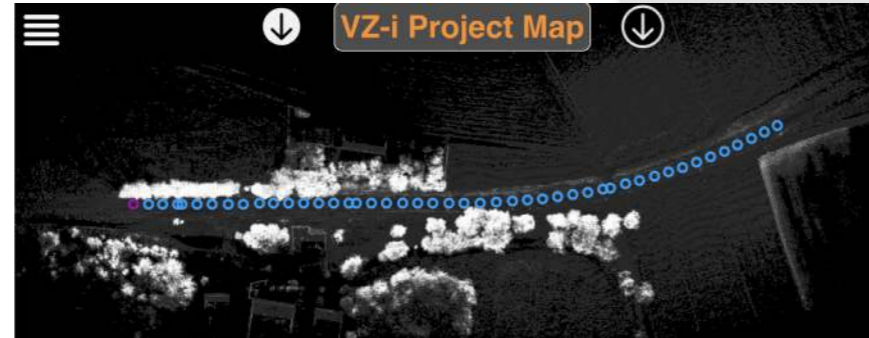
While the scanning platform is still working in the field, the operator can check the registered scan positions and scan data from a remote position via mobile device.
